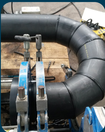
FABRICATION OF SPECIAL FITTINGS
