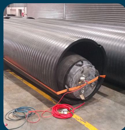
PRESSURE TESTING OF PIPELINES
